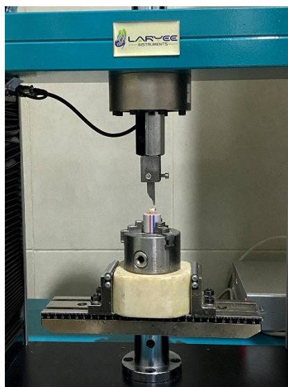
Figure (2): Setup for measuring the shear bond strength of orthodontic brackets bonded to extracted premolars.
